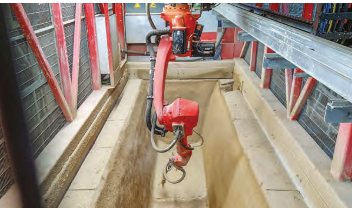
BASILITE QuickStart* is a tundish working lining spray mass to be used on a single, combined, drying and preheating cycle using less energy, less water and delivering higher quality.
