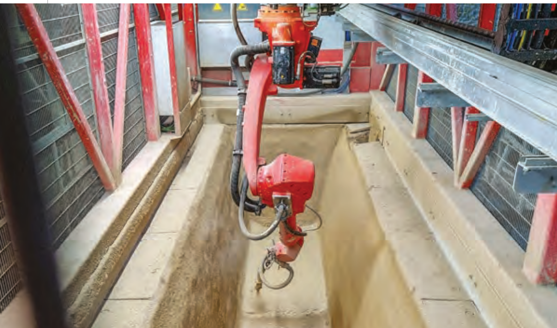
BASILITE QuickStart* is a tundish working lining spray mass to be used on a single, combined, drying and preheating cycle using less energy, less water and delivering higher quality.
